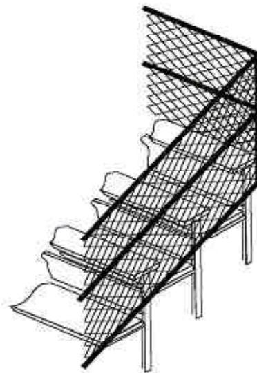
Figure 7: Guardrails with chain link fencing prevent passage of a 4-inch sphere attached to the existing railings
